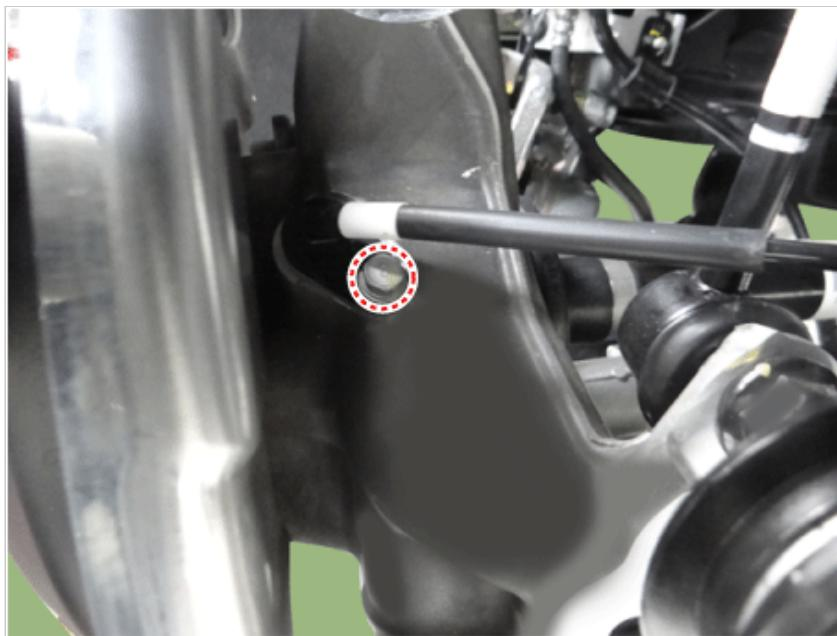
6. Loosen the stabilizer link nut and then separate the rear axle.
