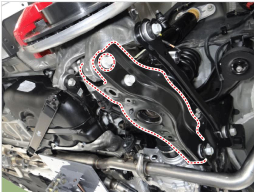
8. Loosen the nut & bolt and then separate the trailing arm from the rear axle.
