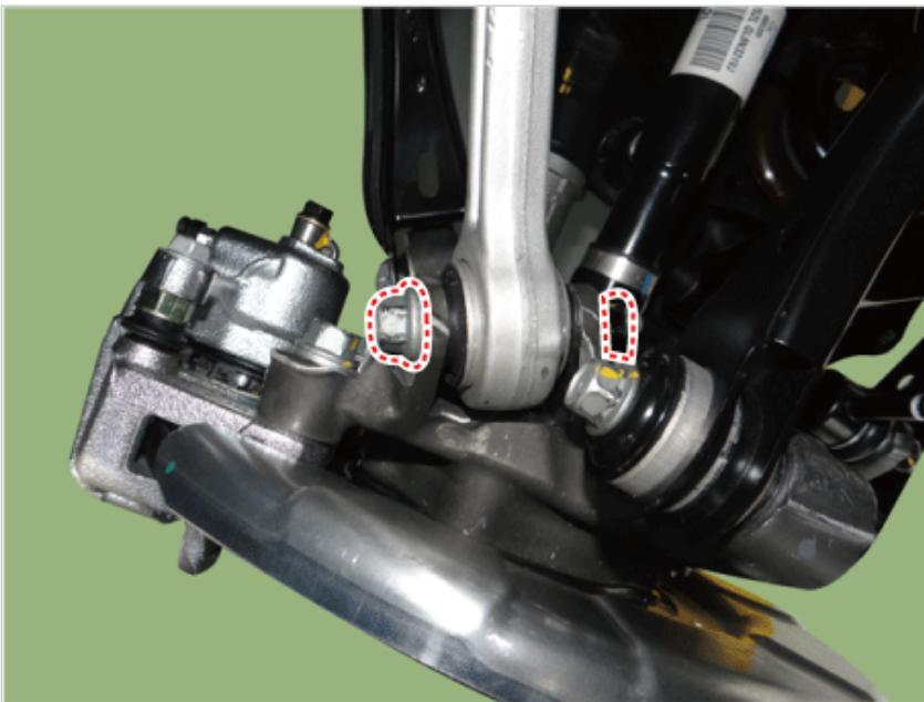
11. Loosen the rear upper arm rear bolt & nut (A) and then separate the rear upper arm rear.
